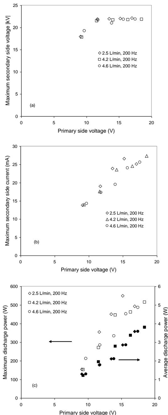
Fig 5. The change in (a) the maximum discharge voltage, (b) the maximum discharge current and (c) the maximum and average discharge power as a function of the primary side voltage for a pulse repetition rate of 200 Hz and air flow rates per electrode of 2.5 to 4.6 L/min.
