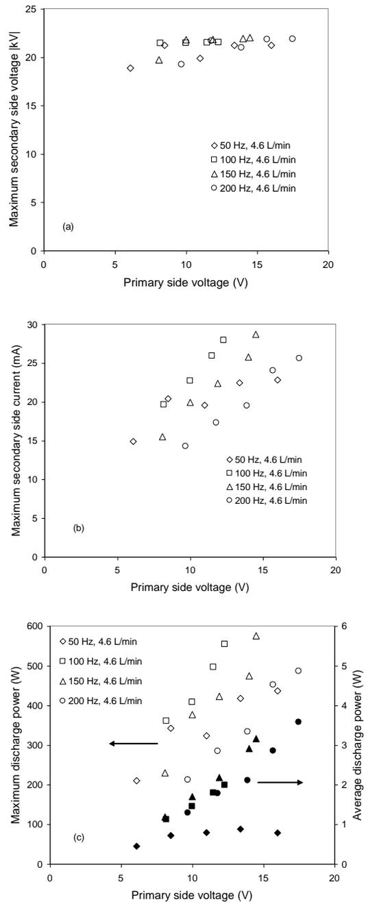
Fig 4. The change in (a) the maximum discharge voltage, (b) the maximum discharge current, and (c) the maximum and average discharge power as a function of the primary side voltage for pulse repetition rates of 50 to 200 Hz and an air flow rate per electrode of 4.6 L/min.
