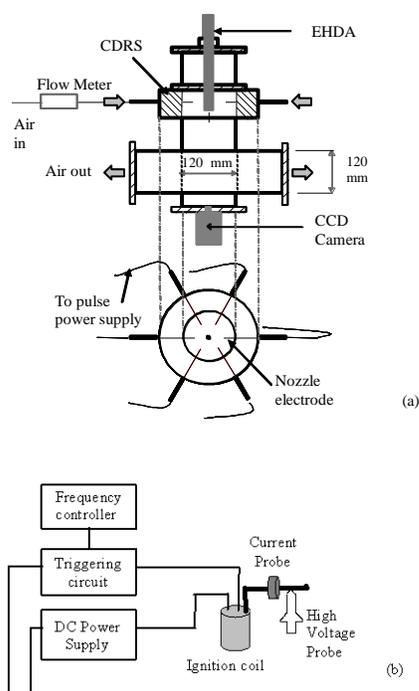
Fig. 1. Schematic of (a) the experimental apparatus used to characterize the RCDRS and (b) the pulse power supply.
