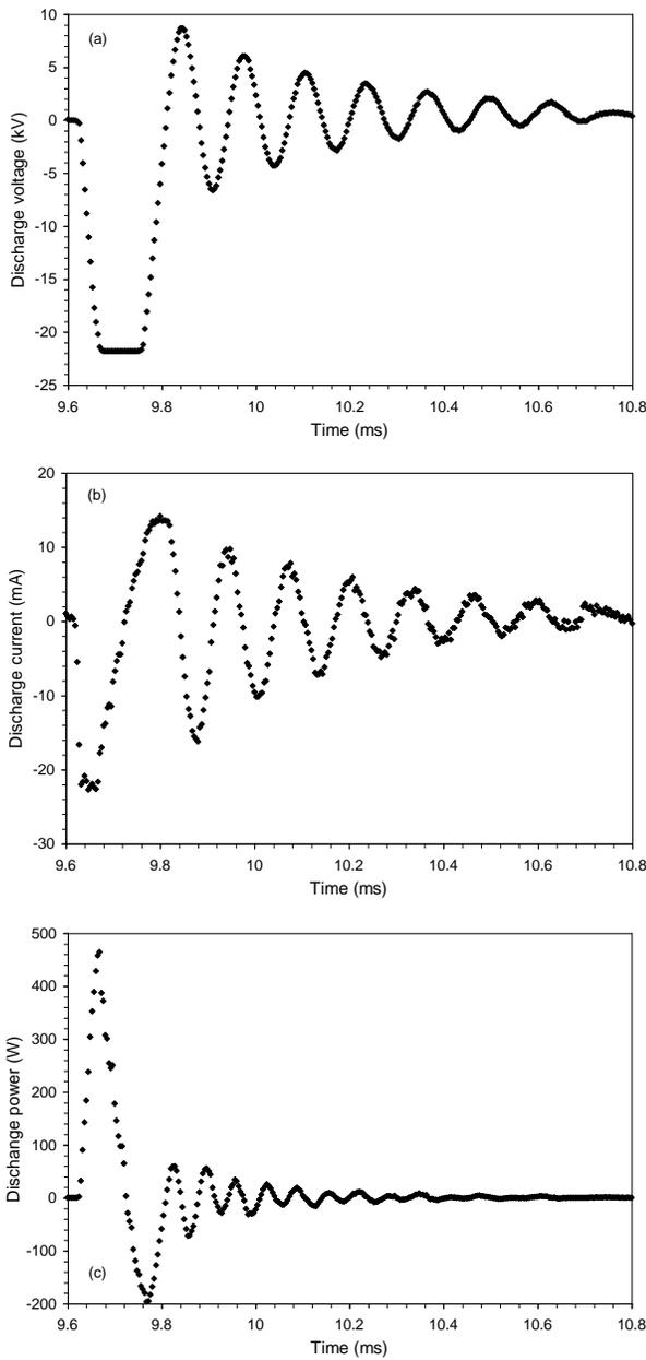
Fig 3. Typical waveforms of the (a) discharge voltage, (b) discharge current, and (c) discharge power from the 6 hollow electrode RCDRS for a primary side charging voltage of 15.7V, air flow rate per electrode of 4.6 L/min and a pulse repetition rate of 200Hz.
