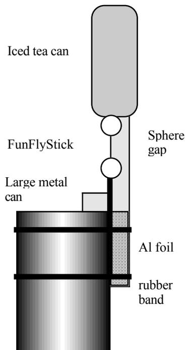
Fig. 5. Iced Tea Can VDG set up for voltage estimate.
