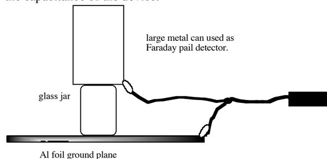
Fig 1. Charge sensor setup
