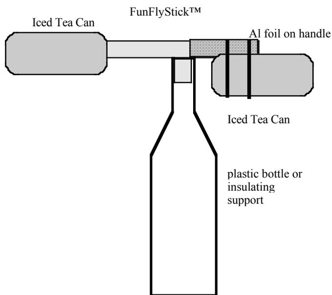
Fig. 7. FunFlyStick™ set up as dipole Van de Graaff generator.
