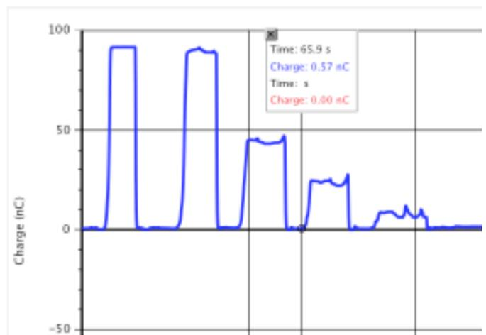
Fig. 4. Charge sensor readings for 1/2, 1/4, 1/8, 1/16, and 1/32 of ITC-VDG maximum charge.
