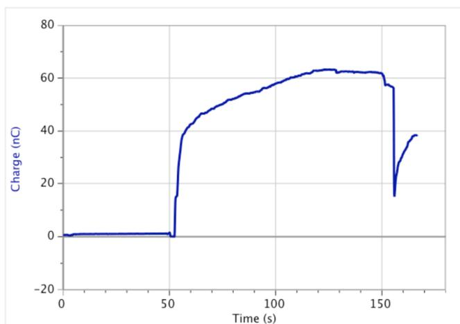
Fig. 6. Sensor graph monitoring charge and spark on ITC-VDG.
