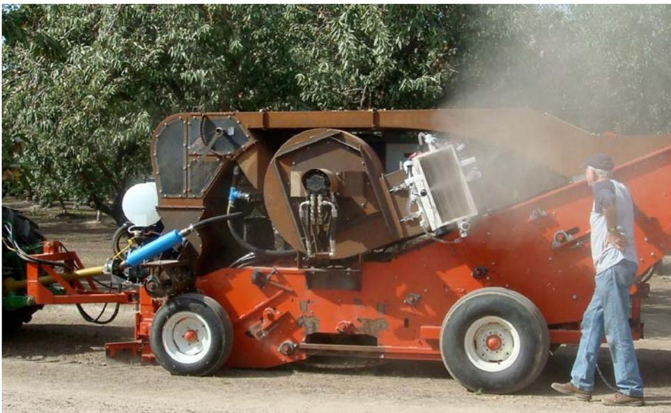
Figure 1. Prototype of nut-harvester with aerodynamic-electrostatic abatement of respirable dust.
