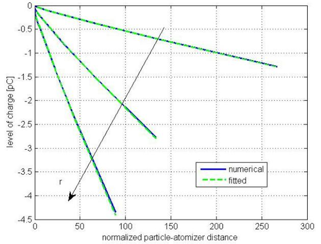
Fig. 7. Comparison of numerical results and fitted data for the value of charge as a function of ligament length ( $r=15, 30, 45\mu\text{m}$ ).
