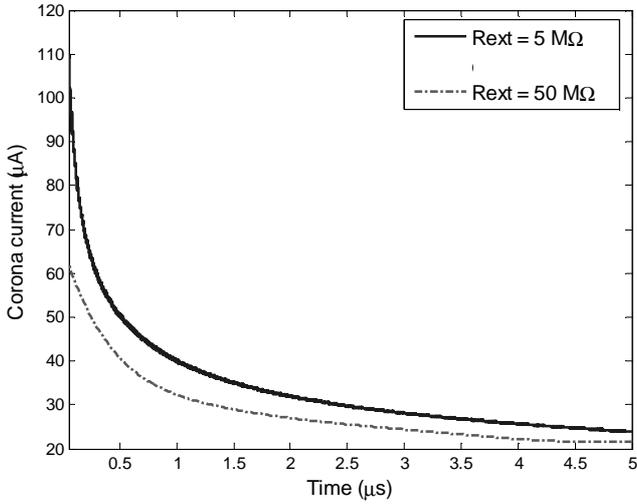
Fig.3. Corona current versus time for two different external resistances ( $V=10\text{kV}$ )
