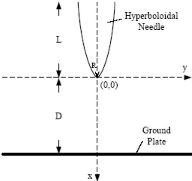
Fig.1. The configuration of corona discharge system.
