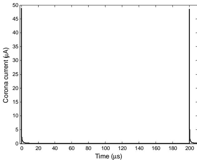
Fig.12. Corona current versus time ( $R_{ext} = 50M\Omega$ )
