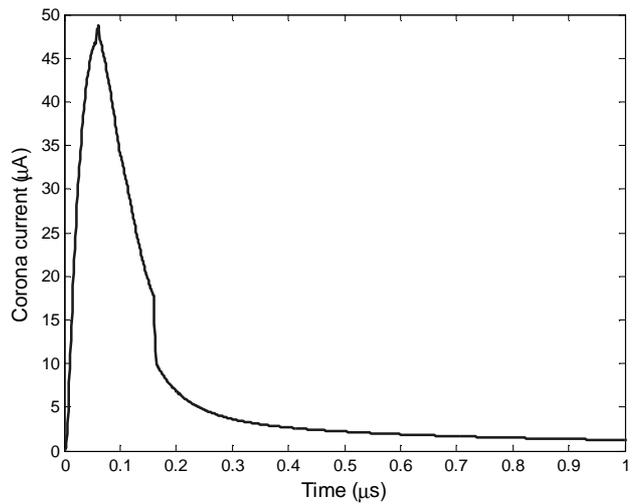
Fig.7. Corona current versus time ( $R_{ext} = 50\text{M}\Omega$ )
