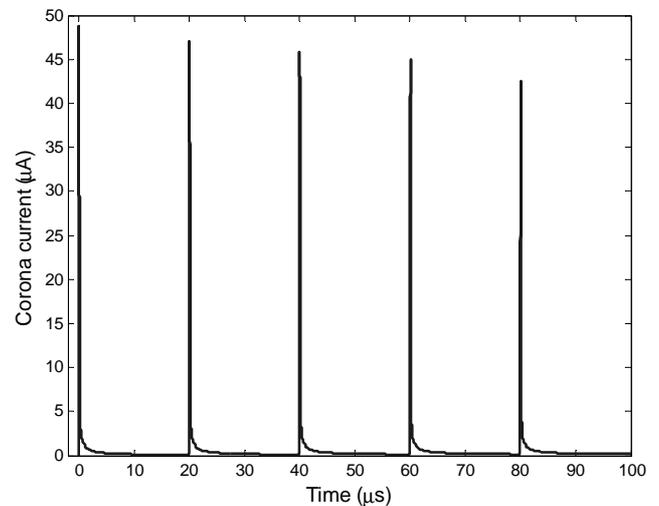
Fig.13. Corona current versus time ( $R_{ext} = 50M\Omega$ )
