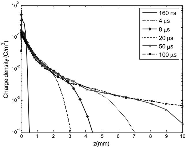
Fig.5. Space charge density along the axis of symmetry at six different instants of time ( $R_{ext}=50\text{M}\Omega$ )
