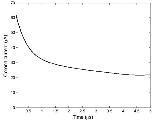
Fig.2. Corona current versus time ( $R_{\text{ext}}=50\text{M}\Omega$ ,  $V=10\text{ kV}$ )
