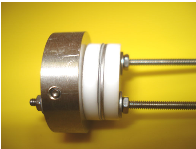
Fig. 3. A photograph of one electrode pair, showing the end cap, the electrode assembly, and two threaded bus lines.
