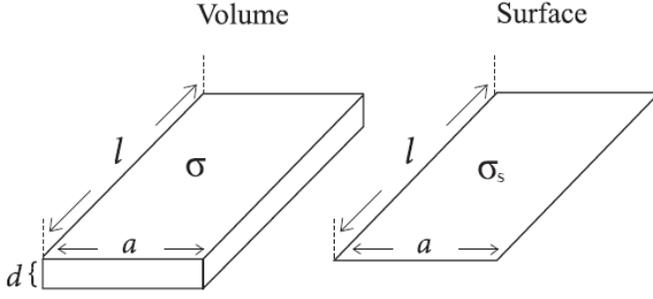
Fig. 2. Volume and surface conductivities for the material and surface layer.
