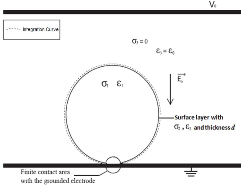
Fig. 1. Conducting spherical particle with surface layer representing moisture, resting on a grounded electrode and exposed to an external electric field.
