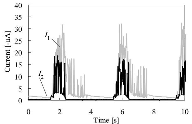
Fig. 13. Waveform of the currents that flow from the metal vessel to the ground obtained when nozzle voltage Type A is applied. The current  $I_1$  is obtained when the water is sprayed.  $I_2$  is obtained when the water is not sprayed.
