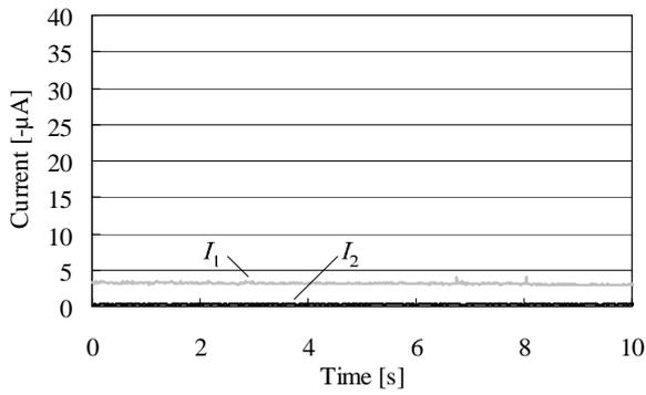
Fig. 14. Waveform of the currents that flow from the metal vessel to the ground obtained when nozzle voltage Type D is applied. The current  $I_1$  is obtained when the water is sprayed.  $I_2$  is obtained when the water is not sprayed.
