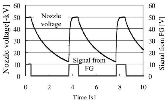
Fig. 11. Nozzle voltage waveform of Type A.
