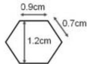
Fig. 3. Mesh size of the conducting net.
