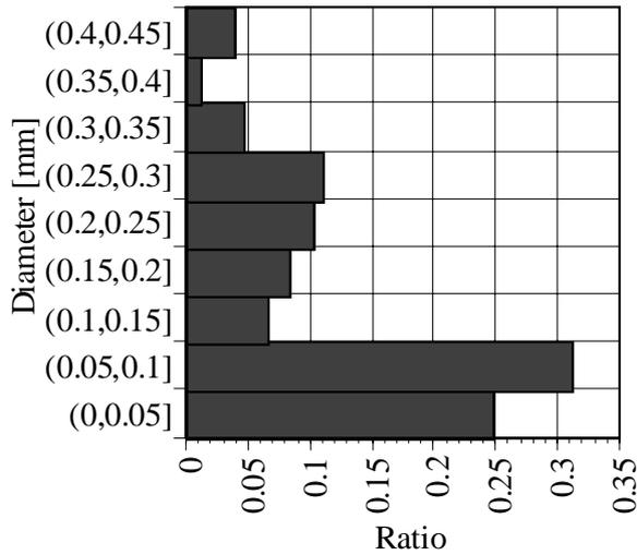
Fig. 4. Droplet-diameter distribution.
