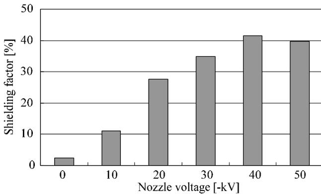
Fig. 8. Shielding factor for various nozzle voltages.
