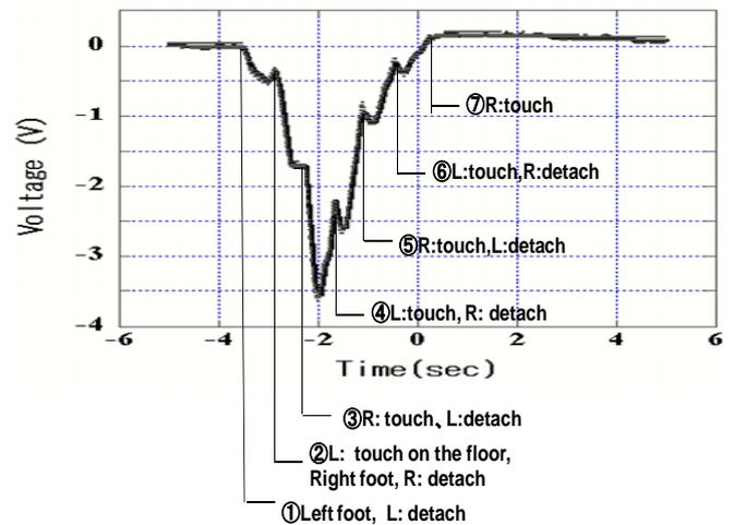
Fig.3 Induction voltage of human body walking under the metal mesh electrode (A: vinyl cloth floor, slipper with rubber sole)
