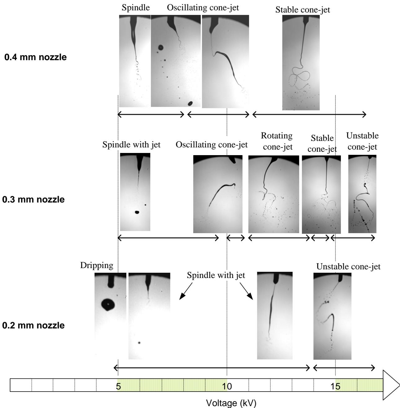
Figure 4. The influence of nozzle diameter on the mode of electrostatic spray.
