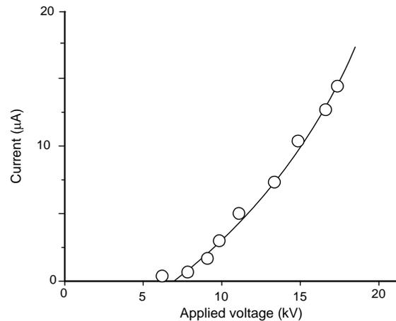
Fig.2 Voltage-Current characteristic of the electro spray with positive polarity (nozzle = 0.3 mm)
