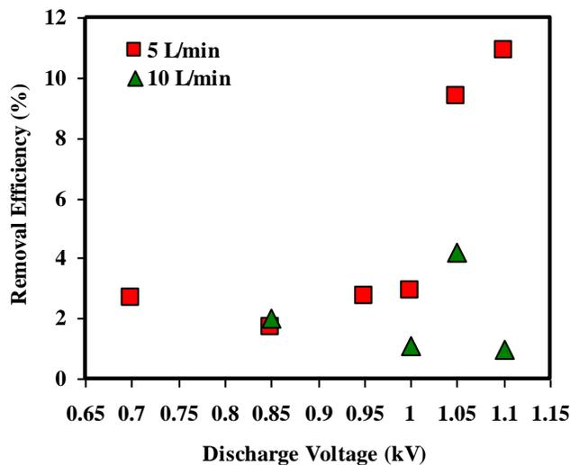
Fig. 8. Removal efficiency of butyric acid versus discharge voltage for air with 58% relative humidity at 5 L/min and 10 L/min.
