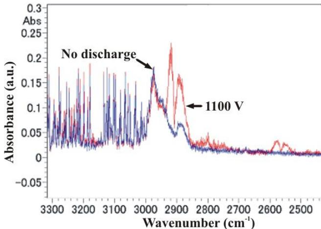
Fig. 12. FTIR spectra of air containing valeric acid and relative humidity of 58% before and after microplasma treatment. Discharge voltage is 1.1 kV. Gas flow rate is set at 2 L/min.
