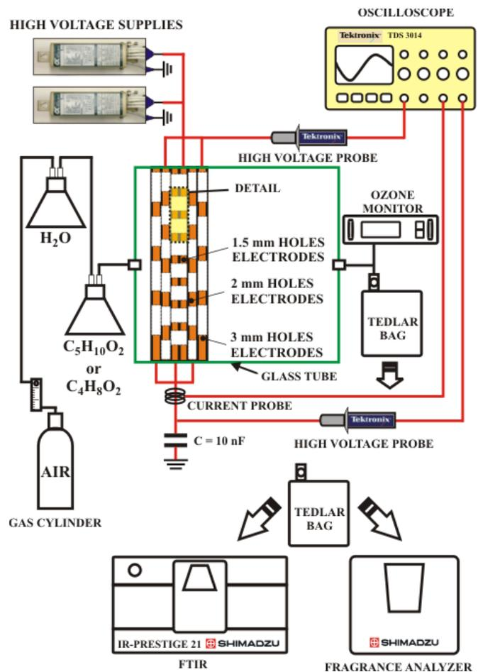
Fig. 1. An experimental setup. Air is flown from a gas cylinder trough a bottle containing distilled water and butyric acid or valeric acid. The treated gas is analyzed by a Ozone Monitor, a Forier Transform Infrared Spectrometer (FTIR) and a Fragrance Analyzer. Microplasma electrodes are powered by two small high voltage power supplies. Two high voltage probes, a current probe and an oscilloscope are measuring the discharge voltage and the corresponding discharge current.
