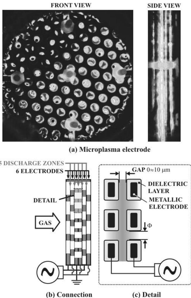
Fig. 2. Microplasma electrode. Photo of the microplasma electrode during discharge (1.1 kV) (a). Connection of electrodes: a honeycomb like structure is obtained by facing together 6 electrodes thus resulting 5 discharge zones (b). Detail of electrode (c).
