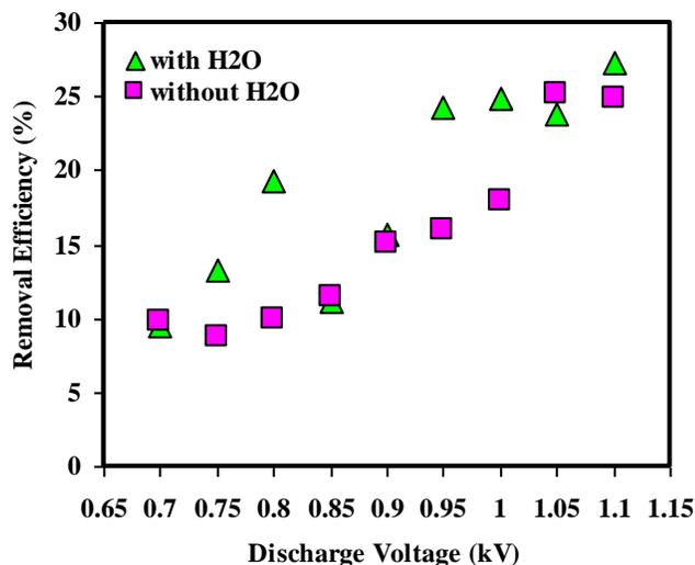
Fig. 7. Removal efficiency of butyric acid versus discharge voltage at a gas flow rate of 2 L/min for dry air and for air with relative humidity of 58%.
