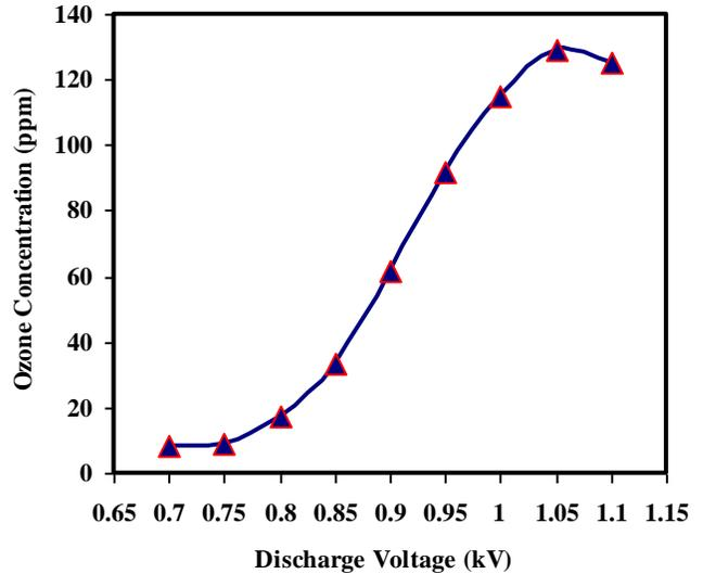
Fig. 13. Ozone generation characteristic versus discharge voltage for air with relative humidity of 58% humidity at 2 L/min.
