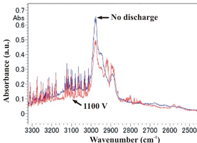
Fig. 10. Spectra of air with relative humidity of 58% containing butyric before and after microplasma treatment at 1.1 kV. Initial concentration of butyric acid is set at 50 ppm. Gas flow rate is set at 2 L/min.
