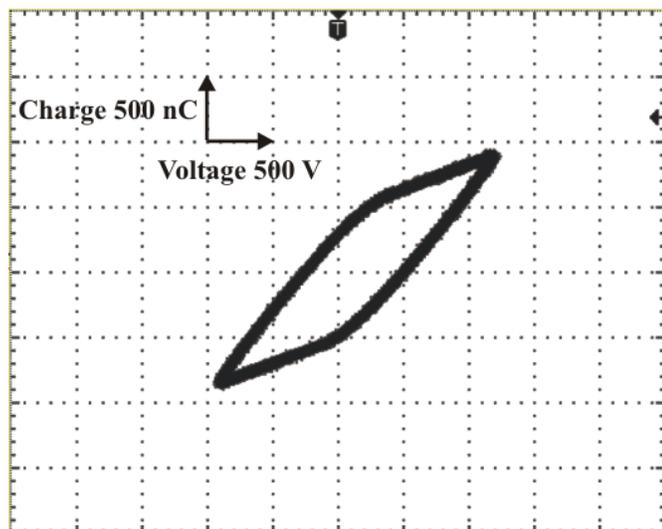
Fig. 4. Lissajous figure represents discharge power of microplasma for electrode arrangement with 6 electrodes faced together at 1.1 kV.
