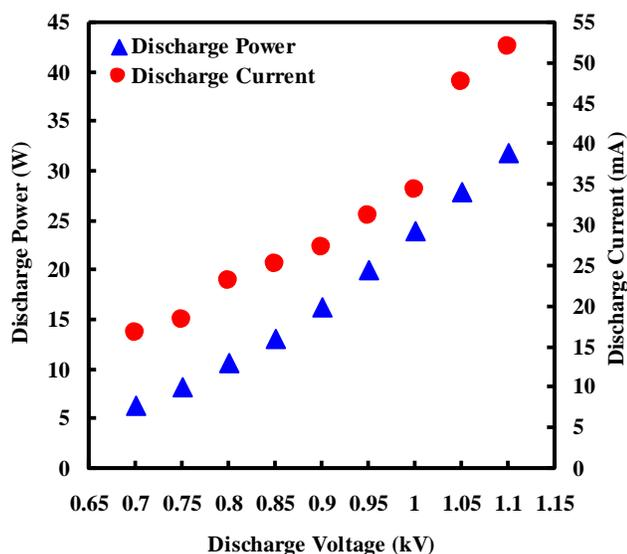
Fig. 5. Characteristic of the microplasma discharge power and discharge current versus discharge voltage for air at 2 L/min.
