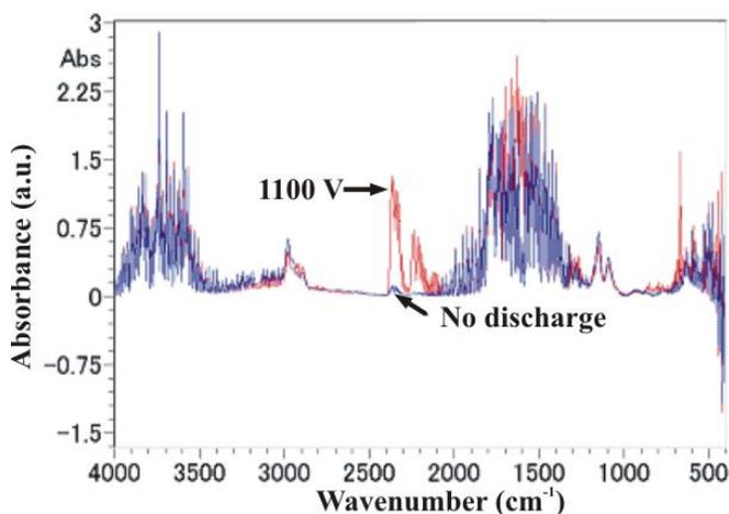
Fig. 6. FTIR spectra of air containing butyric acid and relative humidity of 58% before and after microplasma treatment at 1.1 kV.
