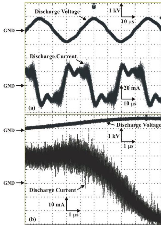
Fig. 3. Waveforms of discharge voltage and corresponding discharge current. Discharge current appeared at steepest slope of discharge voltage (a). Spike currents convoluted in discharge current appeared due to streamers (b).
