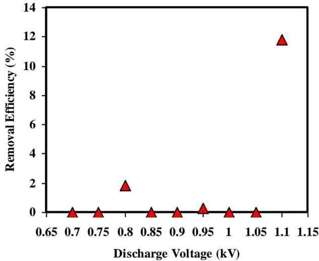
Fig. 11. Removal efficiency of valeric acid versus discharge voltage for air with relative humidity of 58% at a gas flow rate of 2 L/min.
