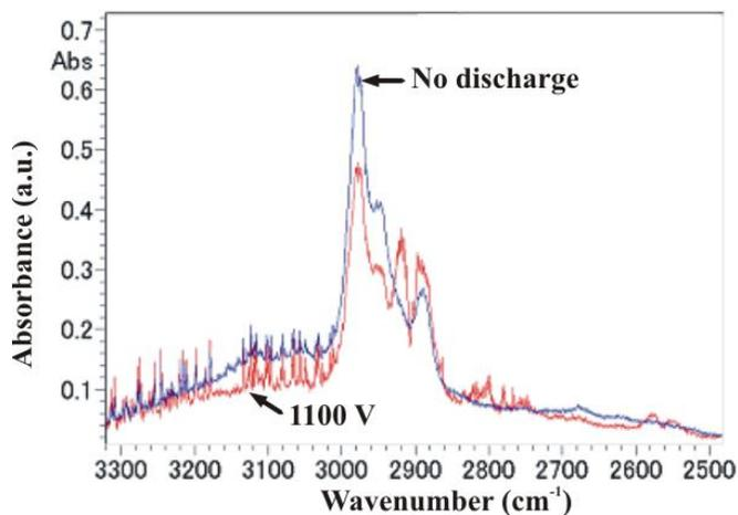
Fig. 9. Spectra of dry air containing butyric acid before and after microplasma treatment at 1.1 kV. Initial concentration of butyric acid is set at 50 ppm. Gas flow rate is set at 2 L/min.
