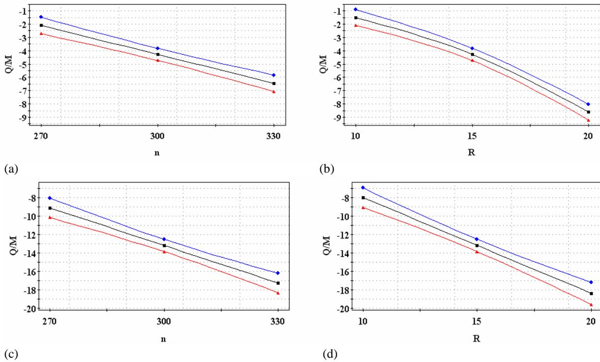
Fig. 7. Predicted charge/mass of ABS (a and b) and HIPS (c and d) granular samples, as function of the oscillation frequency  $n$  [ $\text{min}^{-1}$ ], for a crank length  $R = 15$  mm (a and c), or as function of the length crank  $R$  [mm], for an oscillation frequency  $n = 300$   $\text{min}^{-1}$  (b and d).
