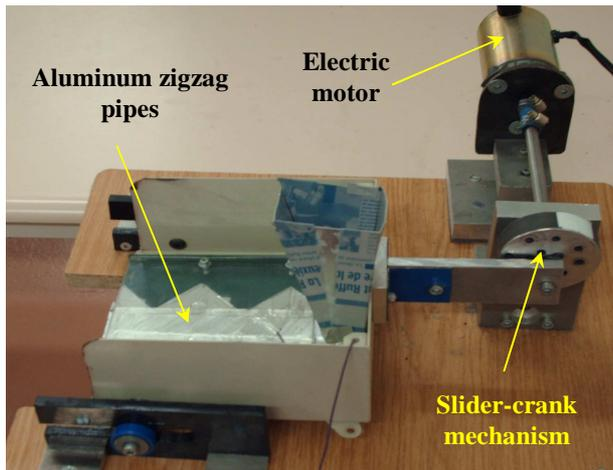
Fig. 2. Vibratory Tribocharging Device.
