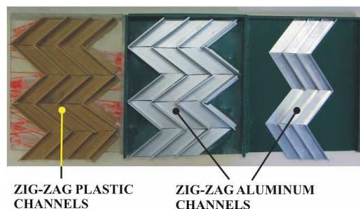
Fig. 1. Zigzag-shaped channels employed as active elements of the tribocharging device. The channels are covered by plate bands of same material, in order to form square cross-section pipes.
