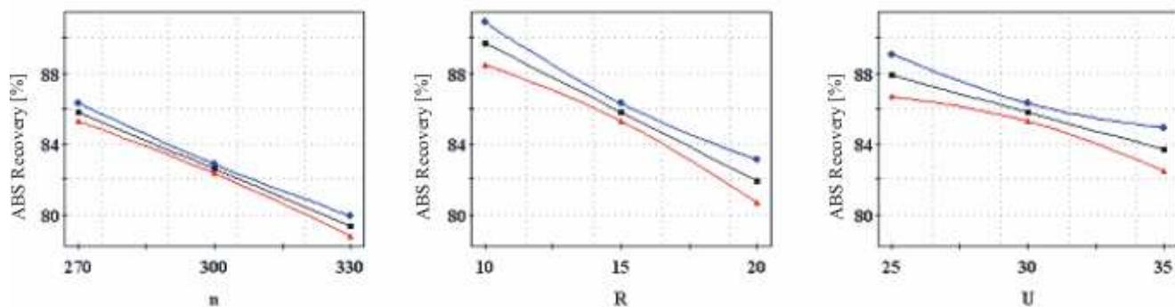
Fig. 8. ABS recovery [%] predicted by MODDE 5.0, as function of the oscillation frequency  $n$  [min<sup>-1</sup>], crank length  $R$  [mm] and applied high voltage  $U$  [kV].
