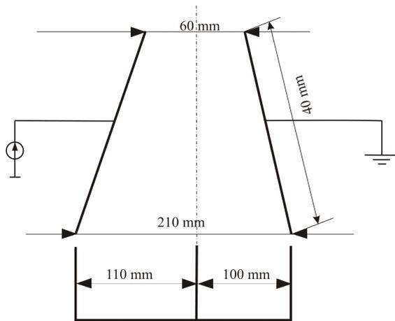
Fig. 3. Configuration of the electrode system.
