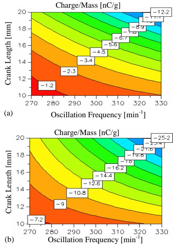
Fig. 6. Contour plots of the charge/mass ratio of ABS (a) and HIPS (b) granular samples, as function of the oscillation frequency  $n$  and the crank length  $R$ .
