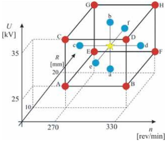
Fig. 5. Composite experimental design for the study of the triboelectrostatic separation of granular plastic mixtures.
